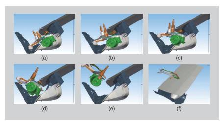
**Figure 2.** A 3-D automotive assembly task that involves inserting or removing a windshield wiper motor from a car body cavity. This problem was solved for clients using the path-planning software of Kineo CAM.
