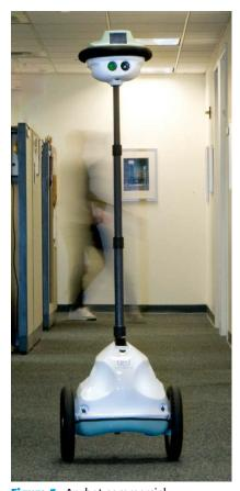
**Figure 3.** Anybot commercial telepresence robot (2010).
