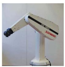
Figure 18. The classic Puma 560 arm is a chain of three rotatable bodies (excluding the end effector) attached to a rigid base. This yields a three-dimensional C-space, which is handled by the standard planning algorithms. (Photo courtesy of the Technical University of Berlin.)
