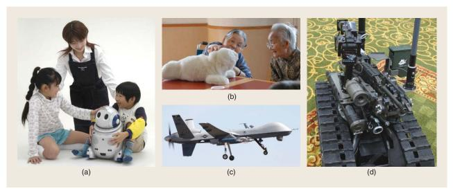
**Figure 1.** Robotic applications of (a), (b) service and (c), (d) combat robots. (a) Childcare robot PaPeRo [32], [73]. [Photo courtesy of NEC Corporation.] (b) Paro therapeutic robot [89]. [Photo courtesy of AIST, Japan.] (c) MQ-9 Reaper Hunter/Killer UAV by General Atomics Aeronautical Systems [33]. (d) Special weapons observation reconnaissance detection system (SWORDS) by Foster-Miller [42]. [Photo courtesy of Foster-Miller.]
