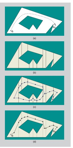
**Figure 5.** A combinatorial planning illustration: a) 2-D polygonal obstacle region with proposed  $q_{\rm l}$  and  $q_{\rm G}$  (one possible solution is shown in a dashed path); b) the trapezoidal decomposition; c) constructing a graph by placing a vertex in every vertical edge segment and every trapezoid interior; and d) connecting  $q_{\rm l}$  and  $q_{\rm G}$  to the graph and searching for a solution path.
