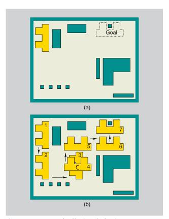
Figure 1. A 2-D example of basic path planning.
