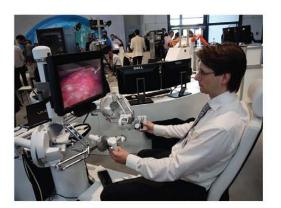
Robotic surgery combines the expertise of surgeons with the precision of robots. Yet for man and machine to seamlessly work together, new interfaces are required that make the robot a natural extension of the surgeon's skills. The MiroSurge robotic surgical system achieves this goal by using a dual sigma.7 haptic interface as both input device and force display.
