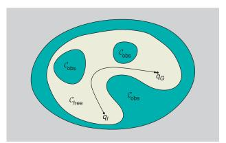
**Figure 4.** In the C-space, the problem looks simple: connect  $q_1$  to  $q_G$  while remaining in  $C_{\text{free}}$ .
